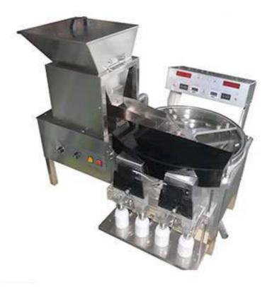
It is a small semi auto electronic desktop quantitative machine. It can count different products such as pills, capsules, tablets, soft gels, sugar, beans and other similar products. Counting different products does not require changing parts on the machine. The Pill Counter has the advantages of fast counting, high precision and simple operation. And the machine is made of high quality stainless steel to avoid contamination of the counting material.
