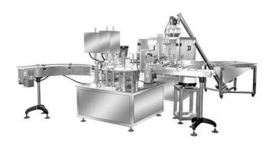
The CapperPacks Rotary Powder Filling Capping Machine is suitable for food salt, sugar powder, cocoa powder, seasoning powder and other powder filling and packaging. It features the screw metering quantifying, rotary positioning filling and the user friendly control system with PLC and touch screen interface.
