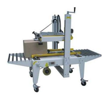
Machine fit for long period single carton size packing, Easy carton size change over. Standard machine height can reach to 600mm more packing range without customize. Machine can be used in many industries. Such as: food industry, medicines, hardware, cosmetics, daily use chemical industry, electronics and furniture.
