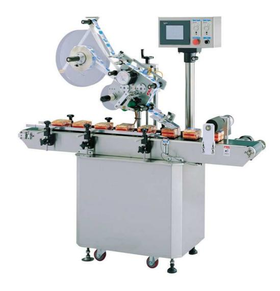
This Machine is designed for top labeling on the flat products. It can be incorporated with a line or operated individually.
