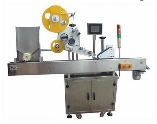
ZHTBW01 horizontal round bottle labeling machine is mainly used for automatic labeling and printing code for bottles with small diameter such as ampoule bottle, vial bottle and oral bottle in pharmaceutical industry.
