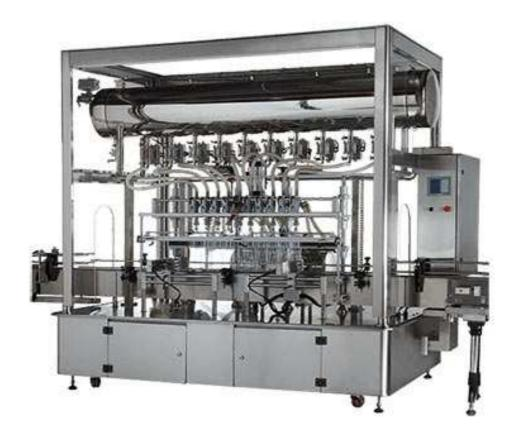
F serials filler provide the same fill level, making them ideal for filling transparent containers that must have a consistent filler level. It is designed to handle for water thin with no particulate liquid.
