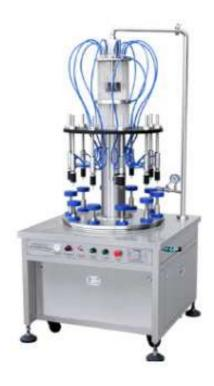
Packry's Rotary Perfume Filling Machine(F-RPFM) is widely used for perfume, fragrance, toliet water and other water-based material, the F-RPFM series utilize fully pneumatic design, apply for those alcoholic liquid material, fully pneumatic can avoid unsafe factor during the whole production. Equip with 10 filling heads and casters, it will improve the filling operation and save labor & space.
