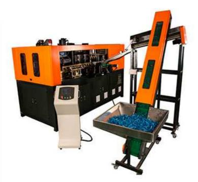
Q series bottle blowing machine can blow different capacities from 100ml to 2000ml. It is suitable for blowing any shape of carbonated beverage bottles, mineral water bottles, pesticide bottles, cosmetic bottles and high temperature resistant bottles made of PET, PP and other crystalline plastics And other packaging containers.
