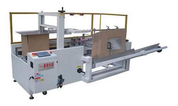
The carton opener is a machine that can automatically shape the carton and seal the bottom tape. The unpacking speed can reach 8-12 boxes/minute, with good quality and affordable price. This box opening machine is widely used in various industries at home and abroad, such as food, medicine, toys, tobacco, daily chemicals, and electronics.
