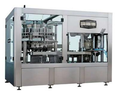
This machine adopts piston filling principle. The machine is equipped with the agitation system and automation system, like three-point level control system, stirring system, No can No filling system and so on.
