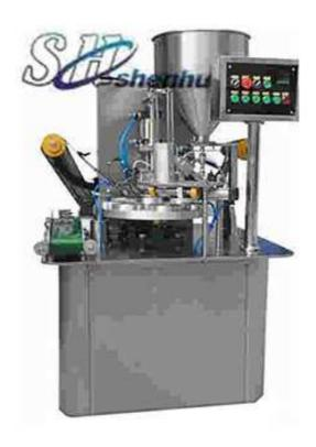
This Rotating disc filling sealing machine is suitable for the production of various kinds of products such as yogurt, water, milk, fruit juice beverage products, automatic cup dropping, filling, absorb film, sealing, automatic box transmission.
