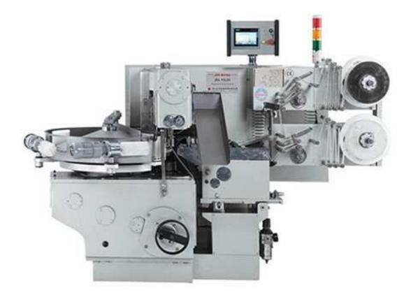
The machine is suitable to wrap dies-formed or deposited sweets of round, oval or oblong shapes. Sweets with semi-liquid centers can be handled without problems. It adopted Indexing drives and cam transfer structure, be able to equip with a sorting station to eliminate sugar dust, chips and broken pieces. An efficient feeding is achieved by the approved plate feeding system. The length of packing material is controlled by the servo motor.
