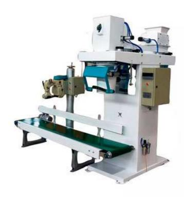
Mainly applicable to powder material (flour, bran, starch, feed, chemical powder etc.) similar materials.
