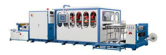
It is suitable to form BOPS, HIPS, PS, PP, PVC, PET, ABS sheet that can produce boxes, trays, bowls, fast-food boxes, dishes and lids etc.
