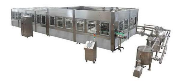
This machine is mainly used in juice and non-carbonated beverage production line. It adopts PLC to control the whole machine operation. Filling temperature automatic setting and adjustable, hot filling technology, if the material temperature not reach the standard the material will be returned back to UHT.
