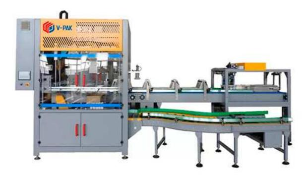
The auto case packer makes the process much simpler and more continuous than manual and semi-automatic carton opening, loading and sealing. For carton sealing, hot melt adhesive tape is used to make the process healthier and the finished carton look much tidier and more beautiful.
