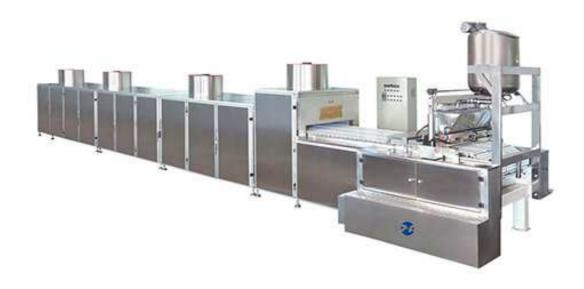
Toffee candy deposting plant suit for producing pure toffee, double color toffee, center filling toffee and stripe toffee with center filling and so on. It gathers machine and electric all in one, using the silicon moulds, and demolding automatically by pneumatic system, with high automation, high output.
