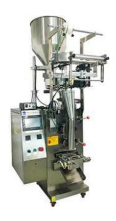
Model XH-20BK is a Rotary measuring cup packing machine for particle food in the market.
