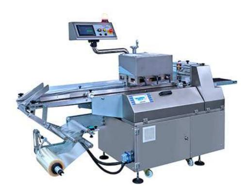
This machine is designed to package single or multi-unit loose, sticky or any product that can not be feed or wrapped by regular Flow Pack Machine.
