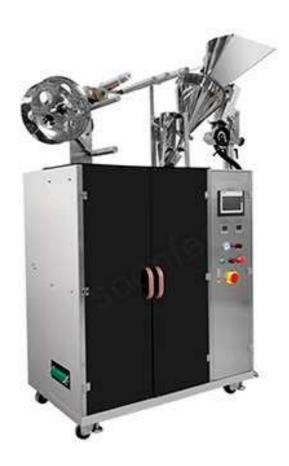
Hanging ear drip coffee bag packing machine. This machine can automatically complete bag making, bag making, measuring, filling, sealing, cutting, counting, printing batch number, and collection.
