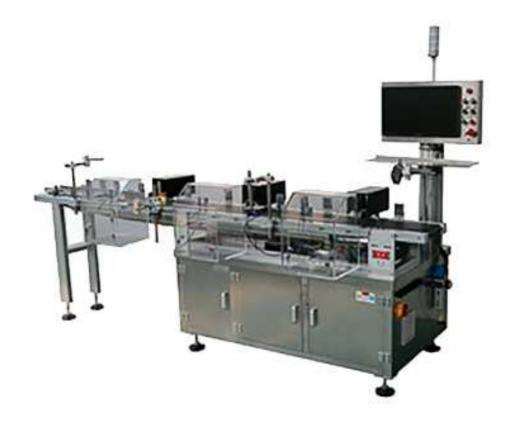
The First-Level Packaging Code Assigned Control System for the first-level packaging of boxed products, the implementation of code assignment, code acquisition, rejection, shunting and other processes.
