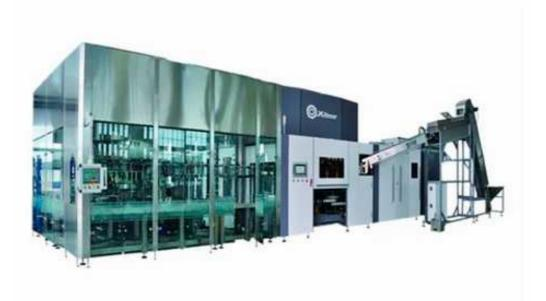
This 12000BPH Blowing Filling Capping Machine's operating interface is simple and easy to understand, and you can switch between multiple languages. It is equipped with an ion precipitator to improve the cleanliness of the packaging container. Multi-layer heating device makes heating more even. The production process is stable and no noise. In addition, it has low production cost and long service life.
