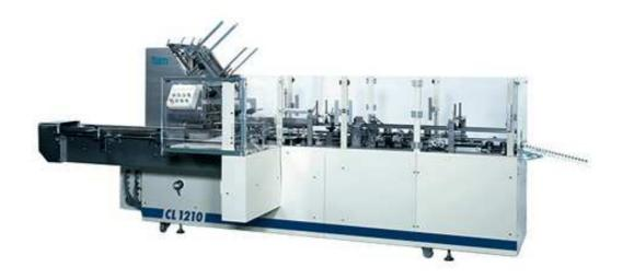
This is our intermittent cartoner designed to handle large boxes. As with the CL810, it too is available with gluing and tucking functions. Size change can be completed in 5 minutes without using tools. Automatic insertion device can be equipped for helping easy filling and for effective streamlining.
