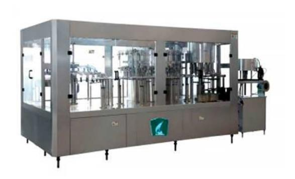
Cola Filling Machine/Cola Filling Production line Description: Material: The material which contact directly with the liquid is the SUS304 (Food grade), made in china. The transmission mechanism and the gear are equipped with firing A4 carbon steel.
