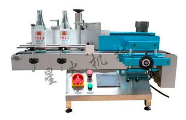
Automatic vertical round bottle positioning labeling machine can be used for cylindrical products and mall cone round bottles circle labeling, front-back two sides labeling semi-circle labeling such as food cans, cosmetic round bottles, and medicine bottles. There are a optional ribbon coder for customers to achieve printing production date info at labeling.
