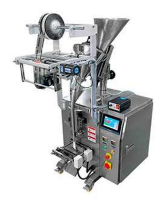
This machine is suitable for packing of sheep milk powder, bean milk powder, cow milk powder, baby milk powder, whole milk powder, etc. It can automatically complete bag—making, measuring, blanking, sealing, cutting, counting, and printing batch number according to customer requirements.
