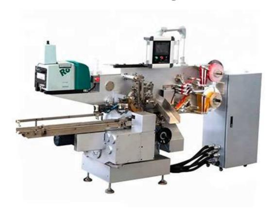
SL-SBZB450D Chocolate Bar Packing Machine is designed for folding packing style, optional single layer and double layer also can be single layer with the label. Packing style available cross fold and envelop fold type. also can pack aluminum foil by changing some parts of the machine.
