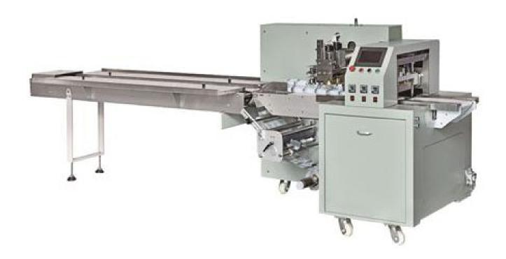
The MK-450XWS flow pack wrapping machine is ideal for a variety of heat-sealable packaging films, with a maximum film width of 450mm. It is designed for packaging regular products like biscuits, soap, instant noodles, and more.
