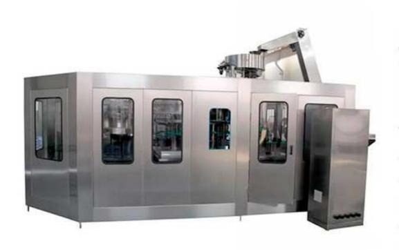
PTPGF 18-6 Carbonated Drink Filling Line For Glass Bottle adopts technology of air conveyor direct connect with bottle infeed starwheel to instead of screw and conveyor. It is easier and more simple to change over bottle size. Adopt neck handling technology to convey bottles. there is no need to adjust the height of equipment and only need to change some spare parts.
