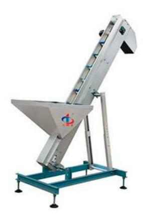
The cap elevator goes with our capping machines in our bottling production line to convey caps to the cap container. The speed of conveying can be adjusted. Inside are sensors which detect when the supply is low. When empty, the sensors stop operation.
