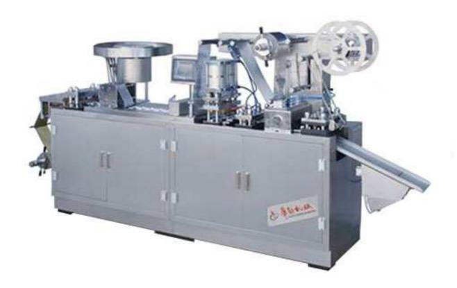
This product adopts international popular materials with good sealing, anti-moisture, protecting from light, using a special cold forming. It is new equipment in the pharmaceutical industry, which will combine both functions, Alu-Alu and Alu-PVC by changing moulds.
