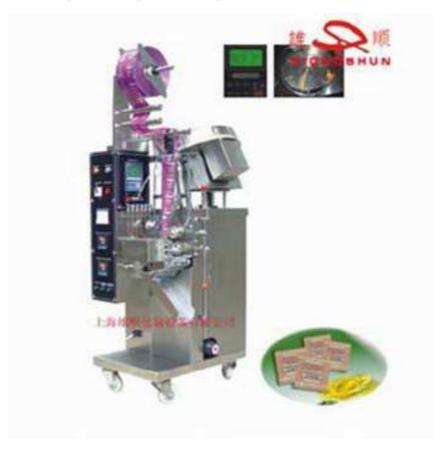
It is suitable for automatically packaging of medicines, foodstuffs, such as round sugar balls etc. Packing material include several kinds of heat-seal lamination, such as PET/plated AL/PE, PET/PE, NYLON etc.
