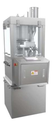
This machine is an intelligent small rotary tablet press. Can be used for pharmaceutical industry R&D centers, laboratories and other small-scale tablet production.
