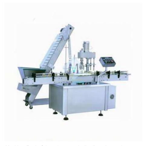
The Cap Sealing Machine (Bottle Crimper) automatically allows for continuous capping of containers using one or multiple crimper heads. It's widely used in capping of metal caps, feeds bottle, places and torques caps. A cap sorting bowl and chute automatically deliver the caps to the containers and star wheel indexing is utilized to move cappers through the capping process.
