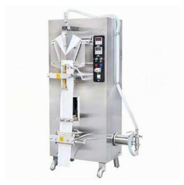
The package machine is suitable for filling soy sauce, vinegar, juice, milk and other liquids, using 0.08 mm polyethylene film, automatic to compete the molding bag, quantitative filling, ink printing, sealing and cutting off process, and film using UV disinfection before packaged, in line with the requirements of food hygiene.
