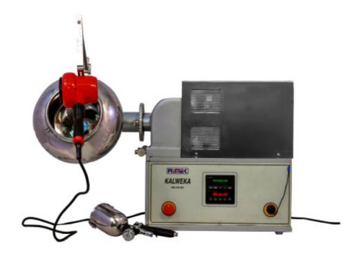
A coating Pan is used for drying coated tablets. It can be mounted on a motor drive unit via universal gearing called UD which permits the coating pan to be held at any angle up to 45° with a reduction in speed. For drying the coated tablets, an infrared drying attachment with adjustable height is provided. The maximum efficient operational capacity is 30% of coating pan volume. Coating Pan-CPS Optional: Heating Accessories, Spray Gun.
