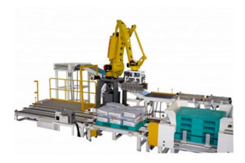
The robot palletizer can be used at any production line, providing intelligent, rogotic and network for production site. It is a palletizing logistic system which can be used in the industry of beer, beverage and foodstuff etc., widely used for carton, plastic crate, bottle, bag, barrel, shrink wrapped product and cans etc.
