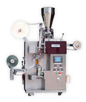
LTDX-115 Tea Bag Packing Machine is a kind of machine used for packing tea seeds, medical, health-care and tea industries granular shaped ingredients. All of these items could be packed with both inner and outer envelops, and with thread and tag at the same time.
