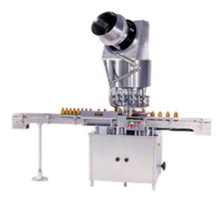
ROPP Capper Machine is used for round or other shape of glass, plastic, LDPE, PET, and HDPE bottles with maximum speed of 240 bottles/min. depends on bottle diameter, height, shape and cap size.
