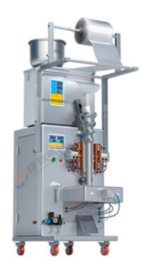
JD produces 200g pneumatic small packing machine suitable for rice millet, cereals, vegetable seeds, cat food and dog food, fertilizer feed, nuts and seeds, corn seeds, coffee beans, coffee powder, flour, pepper, seasoning powder and other particles, powder, material, weighing, filling, sealing.
