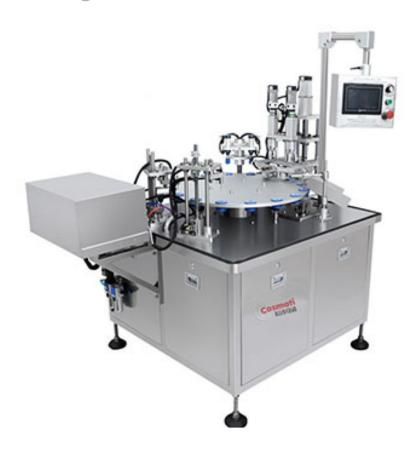
Safety and efficient four head rotary semi-automatic bottle perfume filling machine, pneumatic perfume filler is used for filling floral water, perfume and other water-based materials. The machine adopts negative pressure, suit for fill cologne, and fixed liquid surface type filling. Explosion-proof type products can be provided according to user requirements.
