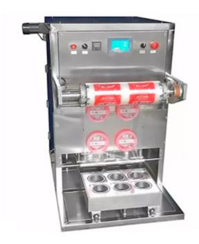
AS-2 Desktop Pneumatic Plastic Cup Sealing Machine is a tabletop model with die cut features. Very compact, it is a drawer style cup sealer that seals and cuts the film around the cup with a pneumatic piston. As you push in the drawer holding your food-filled cups, the sealing film is automatically drawn over the cups and the machine does the rest of the sealing for you.
