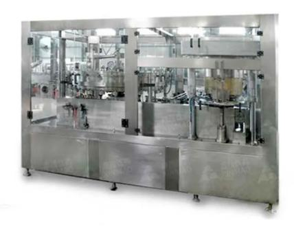
This series of two in one filling machine is used for the production of carbonated beverage, such as Coca Cola, Fanta, Sprite and gas bearing mineral water.
