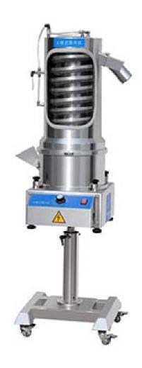
UD220F Uphill Tablet Deduster is a special equipment to wipe out burr and dust of tablet whilst going up way. It can be connected with tablet press and metal detection systems. 316L stainless steel are used for all metal parts contacting tablets.
