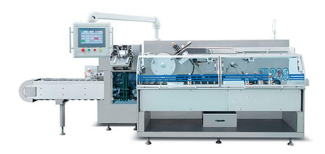
Cartoning machine is a type of packaging machine used to package products into cartons or boxes for transportation and storage.
