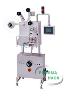
The desiccants strip on the roll holder is routed through several guiding wheels, through the length verification device and into the dispenser. Once the machine starts, the dispenser feeds a preset length of the desiccant strip with the help of the servo motor. If the actual length is confirmed as the setting by the length verification device the desiccant sachet will be cut by the cutter and drop into the bottle via the nozzle.
