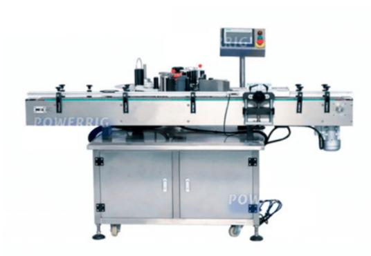
Its production is reasonable. The whole labeling process is automatic, easy to operate, very fast, and the labeling is very consistent, beautiful and clean. It can be used to label round containers in some industries, such as pharmaceutical, chemical and food industries.
