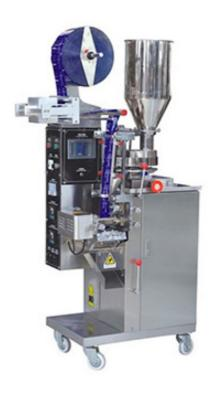
The machine is suitable for packing non sticky, bulk or granular material, such as medical pills, food stuffs, plant seeds, washing powder, coffee, sugar, desiccant etc. The integrated processes of bag making, measuring filling, sealing cutting, counting and hot pressing codes can be done automatically. Packing material include several kinds of heat seal lamination, such as PET/plated AL/PE, PET/PE, PAPER/PE, NYLON etc.
