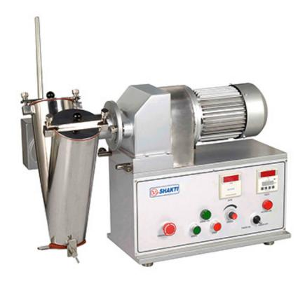
The 'V' Blender is mainly used for mixing of dry power and its provides excellent results when mixing two different powers. This mixer provides a unique movement to the powers and thus mixes them very well.
