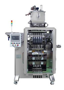
Multi-lane Sachet Packing Machine For Liquid include main filling machines, filler system and elevator that can support many types of bags for packing different kinds of material to your specific demands.
